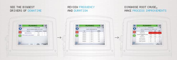
The 1550 and 1650 CLARiTY™ interface presents fault information in a logical way that allows you to identify and focus on the biggest issues and drill down to discover the root causes of unplanned downtime.
